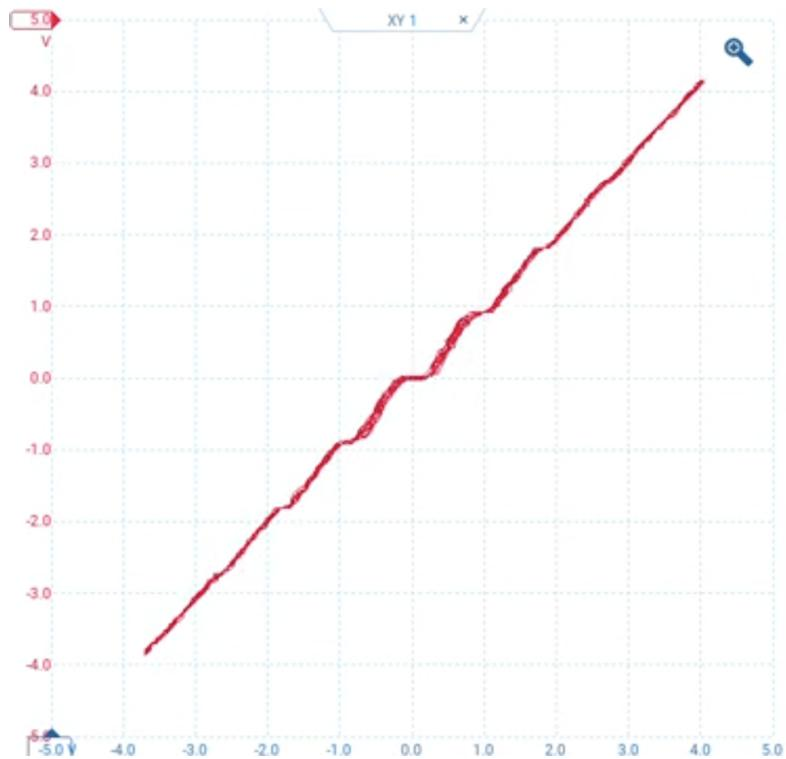
Figure 4: V–I characteristic at  $\sim 77$  K under 44 GHz irradiation showing quantized voltage plateaus (Shapiro steps), confirming the AC Josephson effect.
