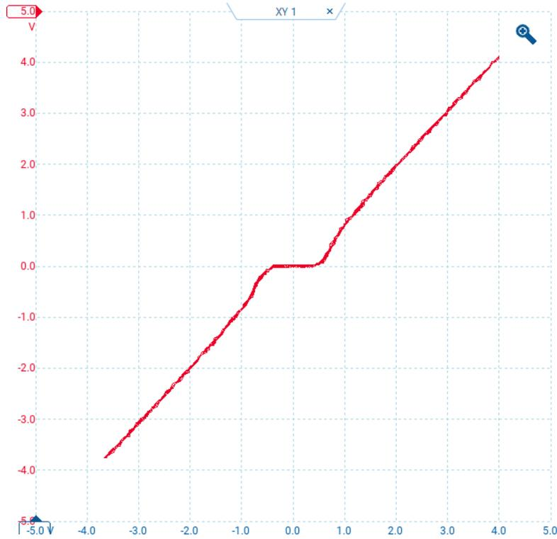
Figure 3: Baseline V–I characteristic at  $\sim 77$  K prior to microwave application. (Horizontal:  $100 \mu\text{A}/\text{div}$ , Vertical:  $100 \mu\text{V}/\text{div}$ )
