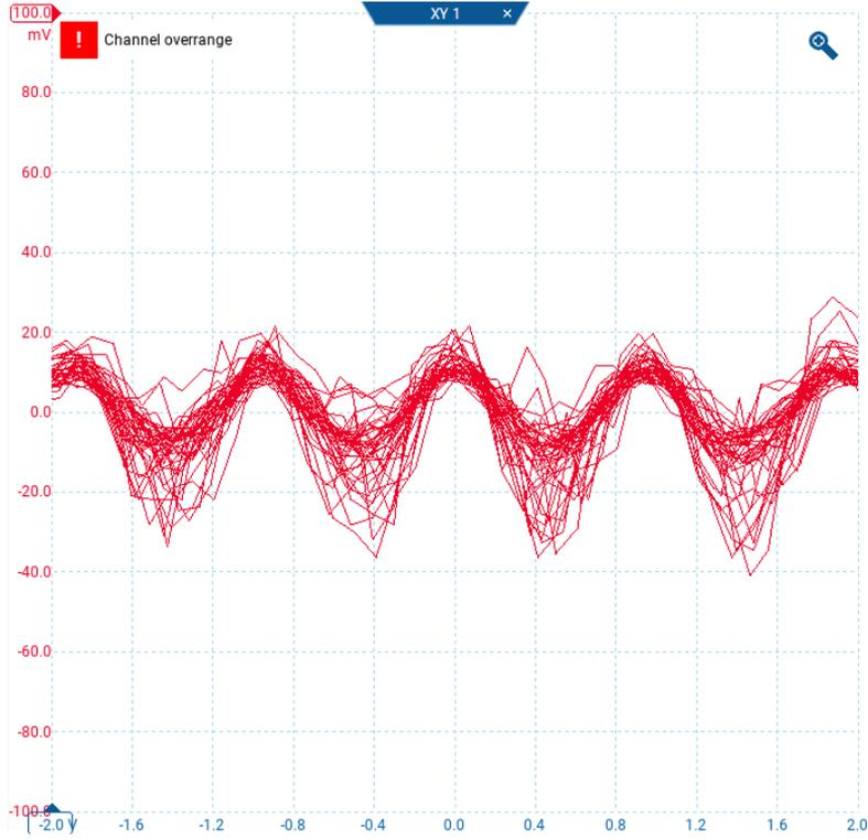
Figure 2:  $V$ - $\Phi$  characteristic of the SQUID at  $\sim 77$  K showing periodic voltage modulation due to magnetic flux quantization. (Horizontal:  $40 \mu\text{A}/\text{div}$ , Vertical:  $20 \mu\text{V}/\text{div}$ )
